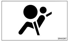
The SRS air bag warning light, displaying 🐉 in the instrument panel, monitors the circuits for the air bag systems, pre-tensioner seat belt system and all related wiring.
