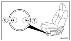
Power adjustment (where fitted): Push each side of the adjusting switch to adjust the seat lumbar area until the desired position is achieved
