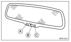
The inside mirror is designed so that it automatically adjusts the reflection according to the intensity of the following vehicle's headlights on the sensor ©.
