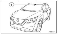
The sensor ① of the rain-sensing auto wiper system located on the upper part of the windscreen, in front of the rear view mirror, can automatically turn on the wipers and adjust the wiper speed depending on the rainfall intensity and the vehicle speed when the lever in the <AUTO> position.
