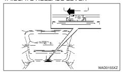
If the tailgate cannot be opened with the power door lock switch due to a discharged battery, follow these steps.
