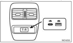
Two USB power ports (where fitted) are provided on the rear of the console box/armrest unit.
