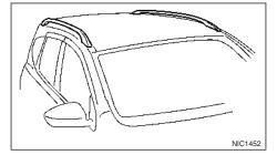
Luggage can be carried on the roof by securing crossbars to the roof rail. Follow all crossbar manufacturers instructions for installing and use of the crossbars. The roof rail is designed to carry loads (luggage plus crossbars) below 75 kg (165 lb). Overloading may cause damage to the vehicle.
