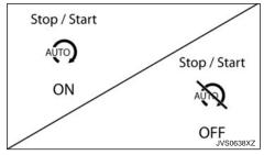
If the Stop/Start System is activated or deactivated using the Stop/Start System OFF switch, the message is shown.
