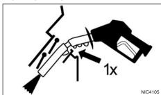
The fuel tank is not equipped with a fuel-filler cap. After opening the fuel-filler lid, insert the fuel pump nozzle directly into the fuel-filler opening and only to the first notch on the bottom of the nozzle When the fuel pump nozzle is pulled out, the fuel-filler opening will be sealed.
