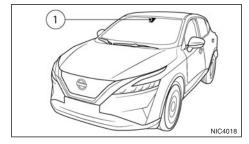
The lane camera unit 1 for the Traffic Sign Recognition (TSR) system is located above the interior rear view mirror. To maintain the proper operation of the Traffic Sign Recognition (TSR) system and prevent a system malfunction, be sure to observe the following:
