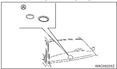
Be sure not to put anything on top of the photo sensor (A) located on the top of the instrument panel. The photo sensor controls the autolight system; if it is covered, the photo sensor reacts as if it is dark and the headlights will illuminate.
