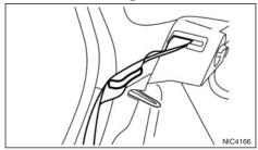
When folding the rear seat forward, the outer seat belts can be stored out of the way using the seat belt hooks as shown in the illustration.
