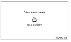
If the system detects that driver fatigue increases or that driver attention is decreasing, the message [Take a break?] appears in the Vehicle Information Display and a chime sounds when the vehicle is driven at speeds above 60 km/h (37 MPH).
