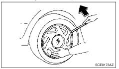
Removing wheel cover (where fitted)
