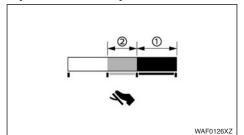
The [ECO Pedal Guide] display can be selected in the vehicle information display in the ECO mode. (See "Vehicle information display" in the "2. Instruments and controls" section.) Use the [ECO Pedal Guidel function for improving fuel economy.
