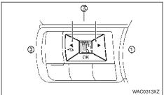
Switches for the vehicle information display are located on the left side of the steering wheel.
