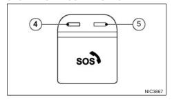
The indicator lights (4) and (5) above the <SOS> button indicate the status of the vehicle emergency call system. If the indicator light is illuminated red or no indicator light is illuminated the emergency call may not connect to the emergency call centre when the <SOS> button is pressed. Also an automatic emergency call may not be sent when a collision occurs.
