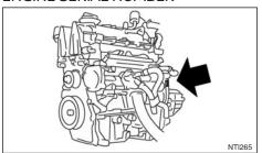
**HR13DDT** engine The number is stamped on the engine as shown.
