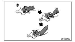
Route the seat belt tongue through the child restraint system and insert it into the buckle until you hear and feel the latch engage.
