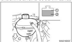
Check the coolant level in the reservoir when the engine is cold. If the coolant level is below MIN level 2), add coolant up to the MAX level (1).
