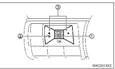
The vehicle information display can be changed using the scroll dial (1), (2) (3), and (4)cated on the steering wheel.
