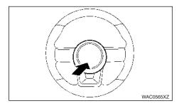
To sound the horn, push the centre pad area of the steering wheel.
