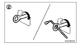
The towing eye is stored with the vehicle tools and located in the spare wheel recess (luggage compartment area).
