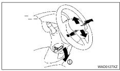
Pull the lock lever (1) down and adjust the steering wheel up, down, forward or rearward to the desired position. Push the lock lever up securely to lock the steering wheel in place.
