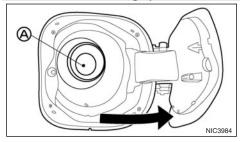
Do not spray high-pressure water onto the capless unit (A) when fuel-filler door is open. Failure to observe this caution may cause the capless unit to malfunction or cause damage to fuel system or engine.
