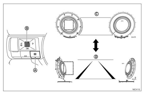
For models with full-screen display, the meter screen view can be changed from Classic View to Enhanced View (D) to expand the vehicle information display area.
