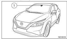
The LDW system will operate when the vehicle is driven at the following speeds and above, and only when the lane markings are clearly visible on the road:
