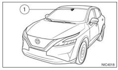
The lane camera unit (1) for the ILI system is located above the interior rear view mirror. To maintain the proper operation of the ILI system and prevent a system malfunction, be sure to observe the follow-
