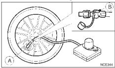
5. Screw the air tube (A) of the compressor securely onto the tyre valve. Make sure that the air compressor switch is in the "OFF" (0) position and the pressure release valve (B) is securely closed.
