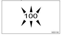
The driver can override ICC by pressing the accelerator. The set speed indicator will flash when the vehicle speed exceeds the set speed. The vehicle detect indicator will turn off when the area ahead of the vehicle is clear. When the pedal is released, the vehicle will return to the previously set speed.
