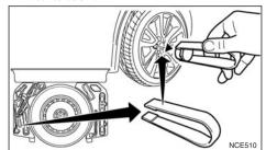
4. Alloy wheels (where fitted): Alloy wheel bolts have a plastic cap that can be removed using tweezers (where fitted) from the tool kit.
