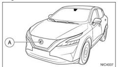
The I-FCW system uses a radar sensor (A) located on the front of the vehicle to measure the distance to a second vehicle ahead in the same lane.
