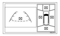
When the "X" icon is displayed on the screen, the camera image may be receiving temporary electronic disturbances from surrounding devices. This will not hinder normal driving operation but the system should be inspected. It is recommended you visit a NISSAN dealer or qualified workshop.
