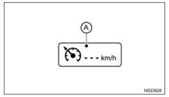
When pushing the ICC ON/OFF switch on, the conventional (fixed speed) cruise control mode display and indicators are displayed in the vehicle information display. After you hold the ICC ON/OFF switch for longer than about 1.5 seconds, the ICC system display goes out. The cruise indicator appears. You can now set your desired cruising speed. Pushing the ICC ON/OFF switch again will turn the system completely off.
