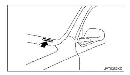
The Vehicle identification number (VIN) is located as shown
