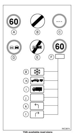
The traffic recognition system displays the following types of road sign:
