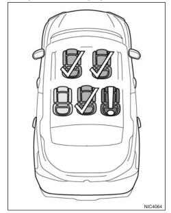
In vehicles fitted with Rear Occupant Detection, in addition to the Seat Belt Warning Light, the Occupant Status Display will be shown in the Vehicle Information Display (See "Vehicle information display" in the "2. Instruments and controls" section) when any vehicle occupant's seat belt is not fastened.
