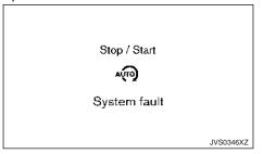
This message is displayed when the Stop/Start System is malfunctioning.
