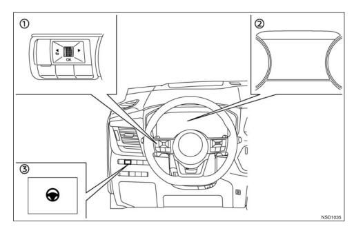
To turn the Steering Assist ON or OFF, push the Steering Assist switch on the instrument panel.
