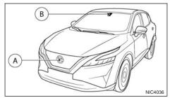
The sensor (A) is located at the front of the vehicle.
