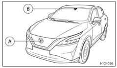
The IEB system uses a radar sensor A located on the front of the vehicle and camera (B) installed behind the windscreen in to measure the distance to the vehicle, pedestrians and cyclists ahead in the same lane (where pedestrian or pedestrian and cyclist detection is fitted).
