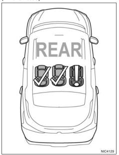
In vehicles not fitted with Rear Occupant Detection, the Rear Passenger Seat Belt Display will be shown in the Vehicle Information Display (See "Vehicle information display" in the "2. Instruments and controls" section) for approximately 65 seconds when the ignition is switched ON while any rear seat belt is unfastened. The driver can acknowledge the display by pushing the **<OK>** steering wheel switch.
