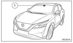
The lane camera unit 1) for the Intelligent Blind Spot Intervention system is located above the interior rear view mirror. To maintain the proper operation of the Intelligent Blind Spot Intervention system and prevent a system malfunction, be sure to observe the following:
