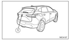
To display the rear view, the Rear-view Monitor system uses a camera ① located just above the vehicle's number plate.
