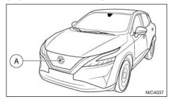
The sensor  $\triangle$  is located at the front of the vehicle. To keep the system operating properly, be sure to observe the following:
