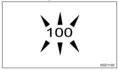
The driver can override ICC by pressing the accelerator. The set speed indicator will flash when the vehicle speed exceeds the set speed. The vehicle detection indicator will turn off when the area ahead of the vehicle is clear. When the pedal is released, the vehicle will return to the previously set speed.
