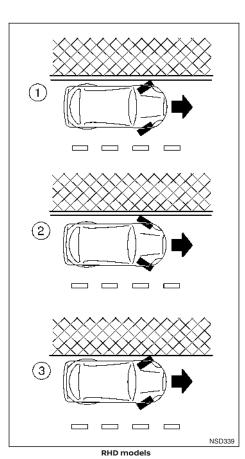
When parked on a sloping driveway, turn the wheels so the vehicle will not roll into the street in case it moves.
