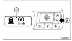
To turn the cruise control on, quickly push and release the ICC switch A. The ICC system ON indicator (grey), and set vehicle speed indicator --- B come on.
