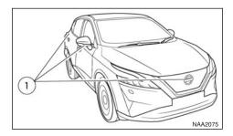
To display the multiple views, the Intelligent Around View Monitor system uses cameras (1) located on the front grille, on the vehicle's outside mirrors and one just above the vehicle's rear number plate.
