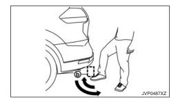
The tailgate can be operated using a quick kicking motion under the centre of the rear bumper.
