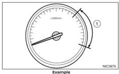
The tachometer indicates engine speed in revolutions per minute (RPM). Do not rev the engine into the red zone (1).
