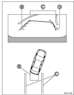
When the vehicle is parked in the space completely, push the P position switch and apply the parking brake.
